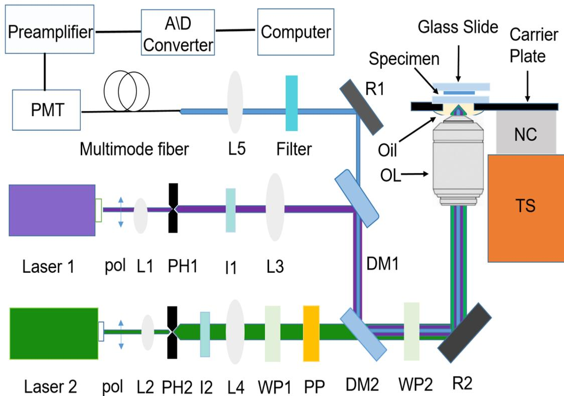
Figure 2.1 A schematic of the STED setup
