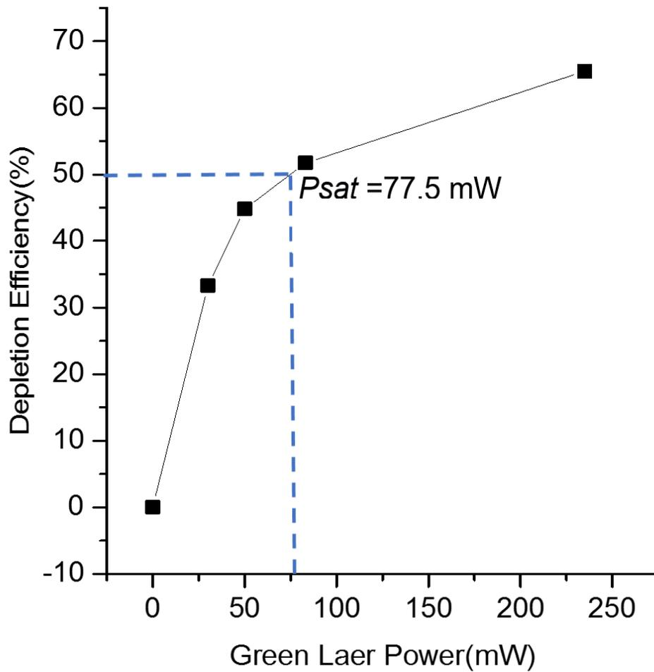
Figure 2.12 STED depletion efficiency as the function of green laser power under excitation of violet laser of 100  $\mu\text{W}$ .
