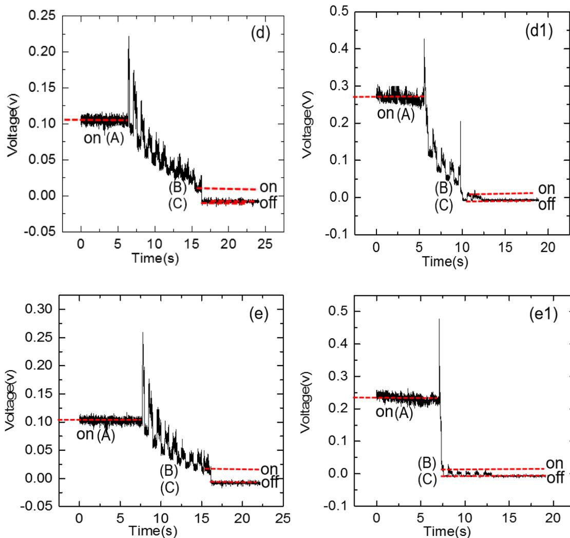
Figure 3.8 Fluorescence intensity using excitation of UV laser of 200  $\mu$ W and depletion of green laser with various powers: (a) and (a1) 50 mW, (b) and (b1) 83 mW, (c) and (c1) 200 mW, (d) and (d1) 287 mW, (e) and (e1) 400 mW; (a), (b), (c), (d) and (e) in the liquid state; (a1), (b1), (c1), (d1) and (e1) in the solid state.
