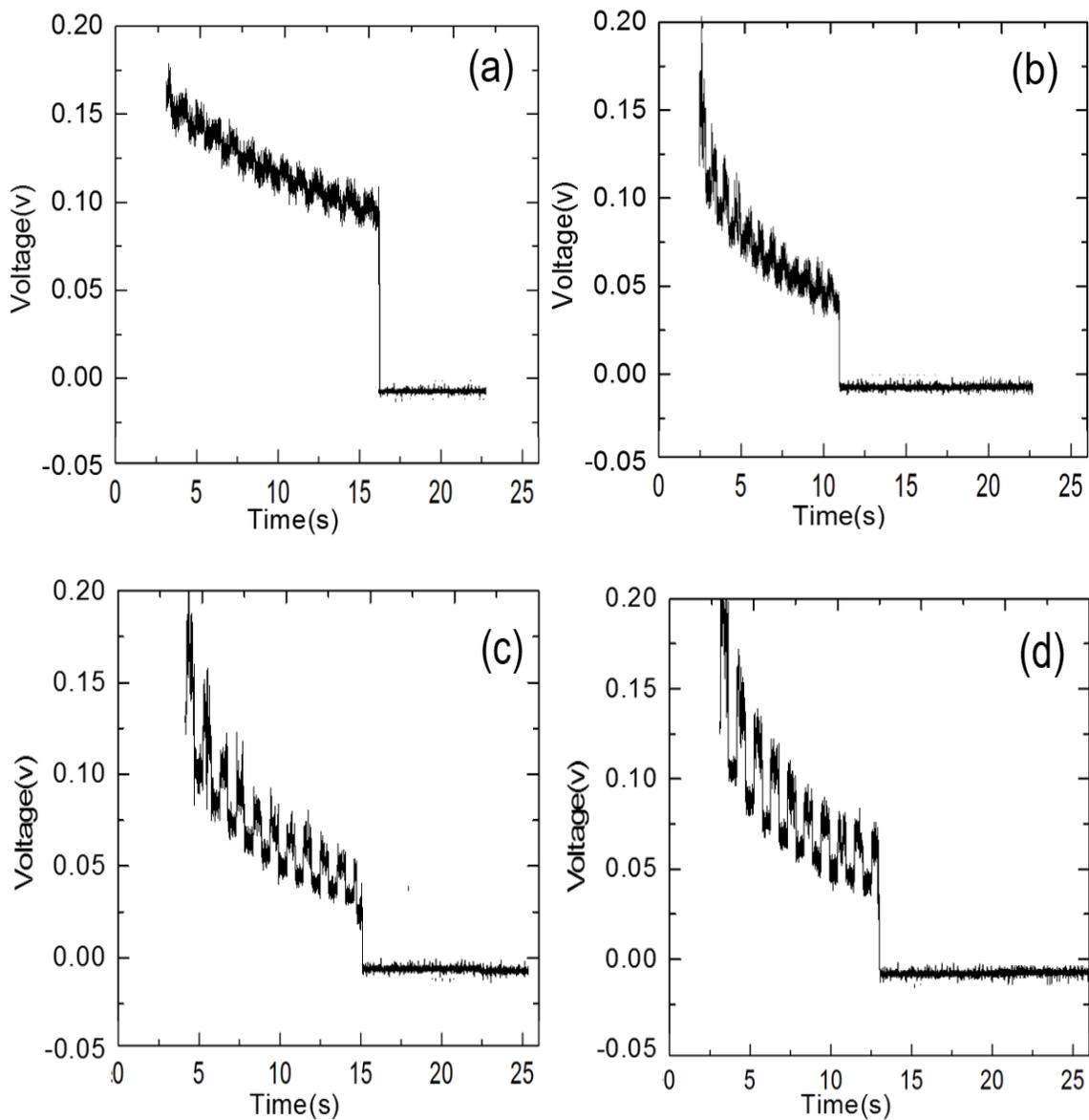
Figure 3.7 Fluorescence intensity using excitation of UV laser of 100  $\mu$ W and depletion of green laser with various powers 100  $\mu$ W and depletion of green laser with various powers: (a) 50 mW, (b) 83 mW, (c) 287 mW, (d) 402 mW.
