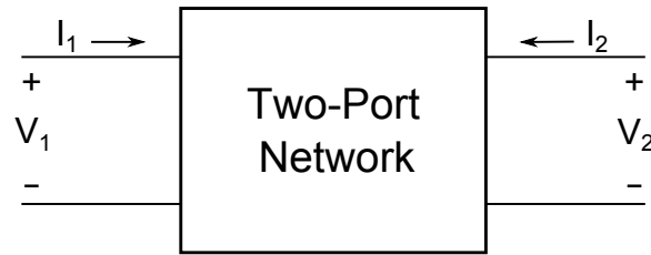
Fig. 2.2. A schematic representation of a two-port network.
