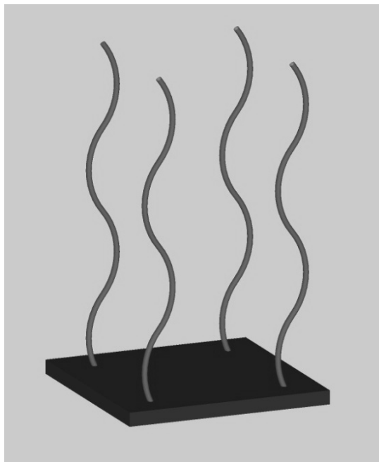
Figure 1.2 – Surface of an implant (black) coated with hydrophilic polyethylene glycol chains (gray) used for anti-fouling. The polyethylene glycol chains attract water molecules which form a barrier between the biological system and the surface of the implant [7].
