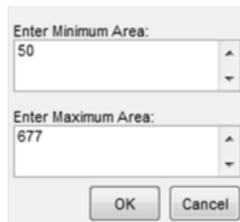
Figure 3.19 – The 'Filter' function was designed to allow the user to filter out cell areas by utilizing the desired minimum and maximum areas. The areas are in terms of pixels.
