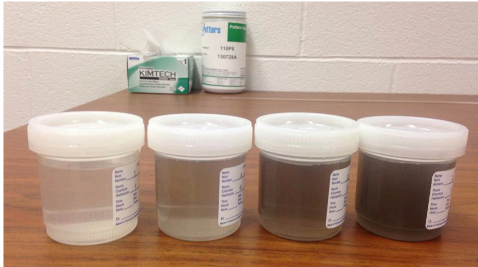
Figure 11: phantom solutions of Luxsil microspheres
