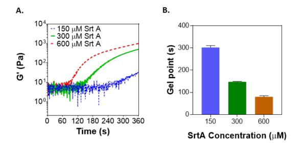
Fig. 4.4. (A) In situ rheometry of PEG-peptide (2 wt%,  $R_{GGGG:LPRTG} = 1$ ) hydrogel crosslinking. G" omitted for clarity. (B) Gel points were calculated by determining the initial time point at which G' was greater than G".
