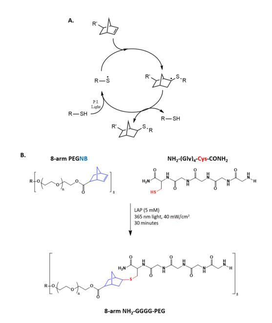
Fig. 1.4. Schematic representation of (A) thiol-ene step growth polymerization and (B) thiol-ene-mediated conjugation of pendent peptides to 8-arm PEGNB.
