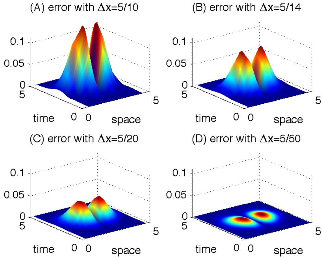
Figure 5.3: Numerical error (5.4) with decreasing stepsizes  $\Delta x$ .
