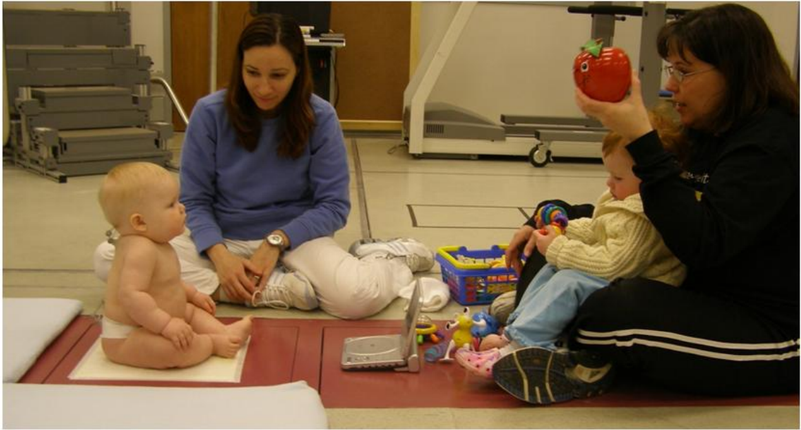
Figure 6.1. Postural sway COP data is collected as an infant sits on a force plate. COP data was used to train the neural network.
