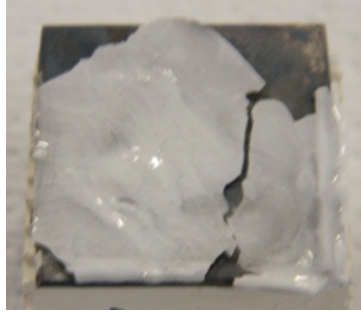
Figure 11 Alumina adhesive + silica + sodium silicate sample failure during curing
