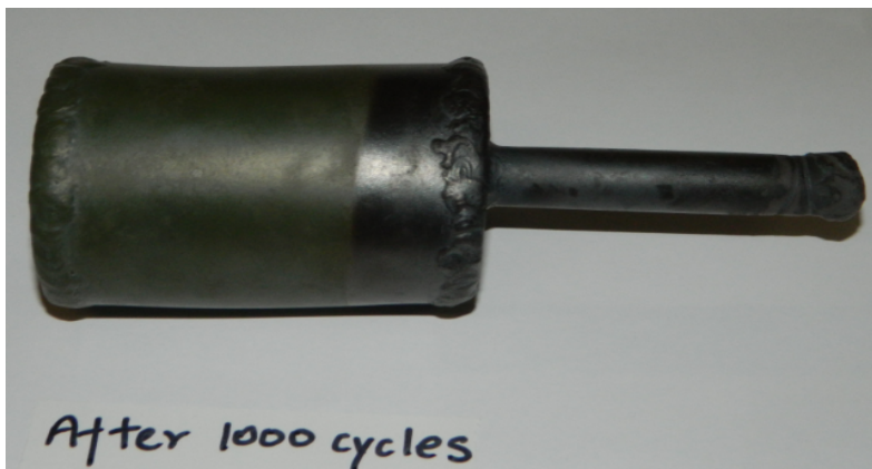
Figure 28 Sealed cylinder after 1000 cycles in aerobic conditions
