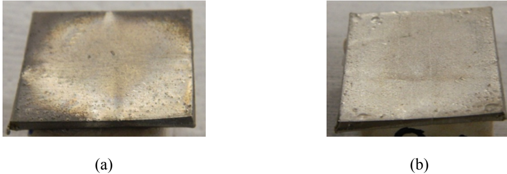
Figure 15 Electroplated nickel sample (a) Before testing; (b) After testing
