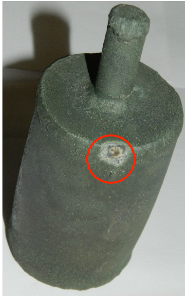
Figure 37 Electroplated Ni cylinder B (150 \mu\text{m} of electroplated nickel) after 100 cycles and the point of failure
