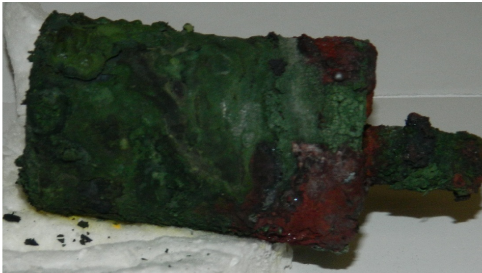
Figure 41 Chrome-plated cylinder (150 \mu\text{m} ) failed after 3 thermal cycles
