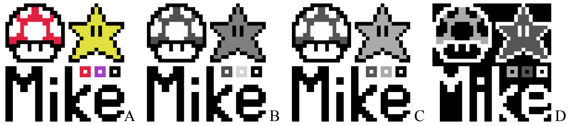
Figure B.2: Visual representation of data conversion in MATLAB in preparation of printing. The data can be imported as a color bitmap image (A). From there, it is converted to grayscale (B) and down-sampled to 2 bits (C). The final step is a polarity inversion (D). (Mushroom and Starman are fair-use images which may be subject to copyright by Nintendo Co., Ltd.)
