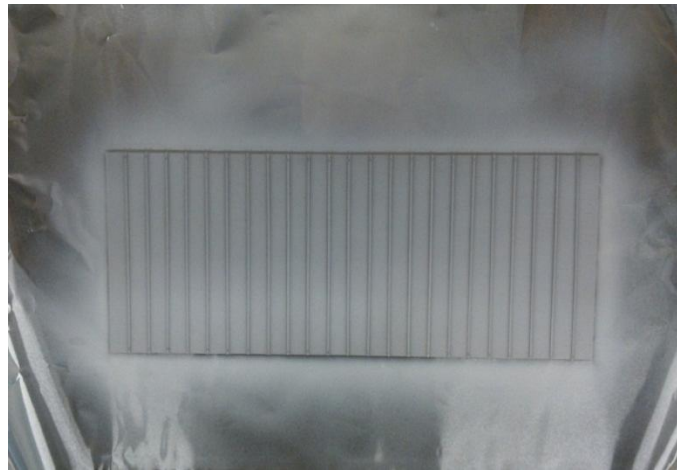
Figure 4.7 TiO 2 photocatalyst was sprayed on the transverse No.1 rough plate
