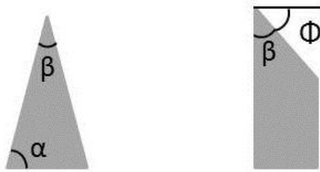
Figure 3.9 Isosceles triangle and chamfer shape of roughness
