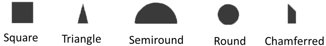
Figure 3.3 Five different shapes of the roughness element studied in this work
