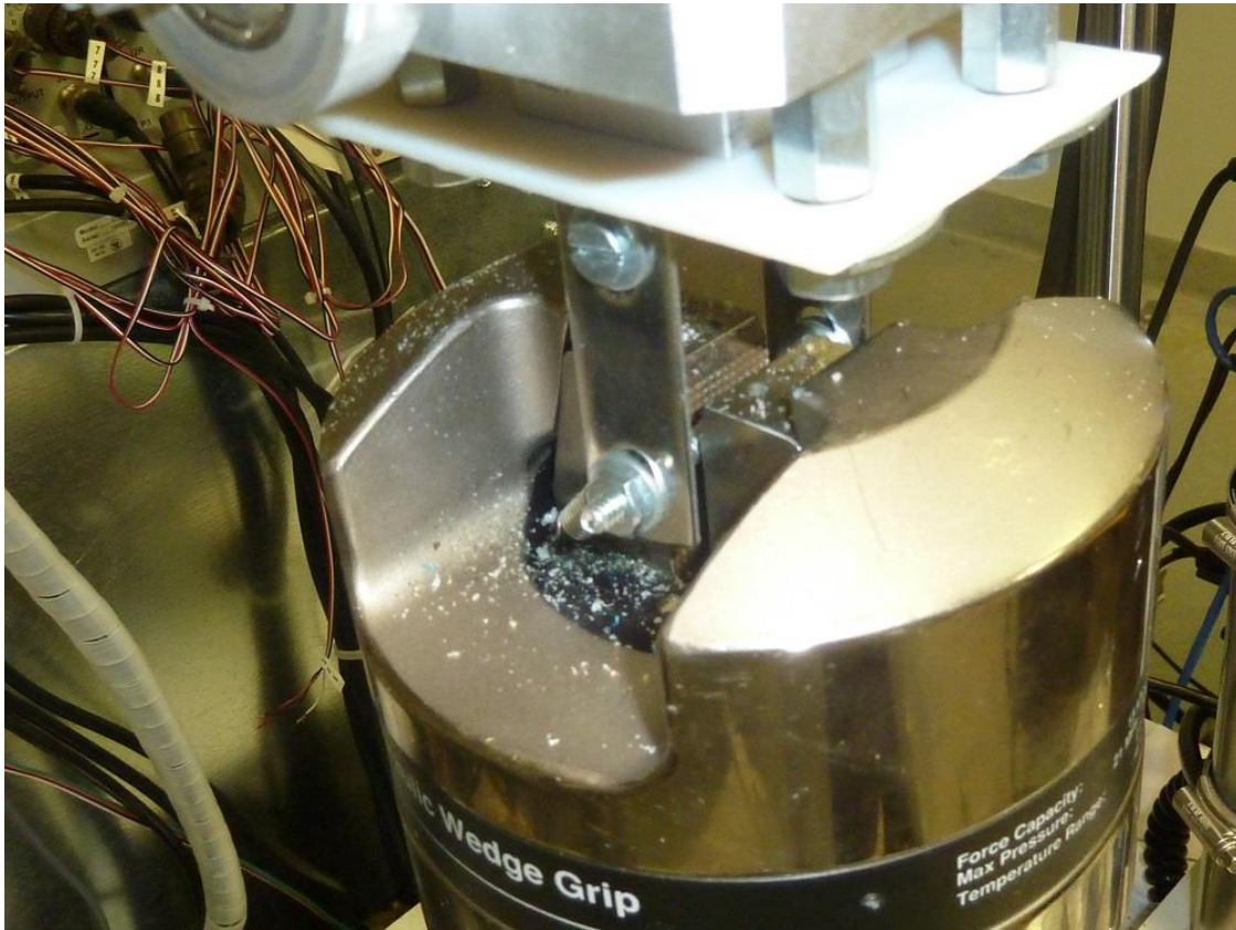
Figure 3.20. Hydraulic clamp grips onto one end of coupler. The other end of the coupler is attached to a pedicle screw (not shown).
