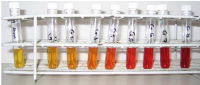
Figure 2.1 Current visual detection method for hemolyzed samples. From left to right, ranks pure to grossly hemolyzed samples, with free hemoglobin in plasma ranging from less than 0.5 g/dL to greater than 30g/dL [16].
