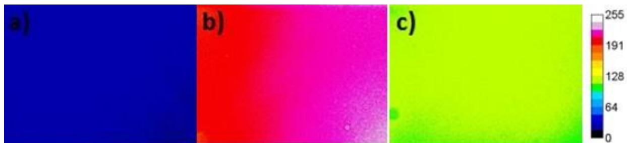
Figure 3-4. MEF results when sputtering a silver layer. a) is the control group without silver (identical to sputtering 90 seconds), b) was sputtered with silver for 180 seconds, and c) was sputtered with silver for 270 seconds.
