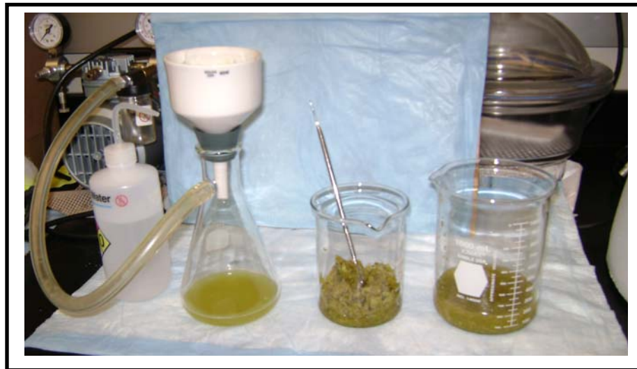
Figure 6.2 Cactus pad preparation showing vacuum filtration apparatus
