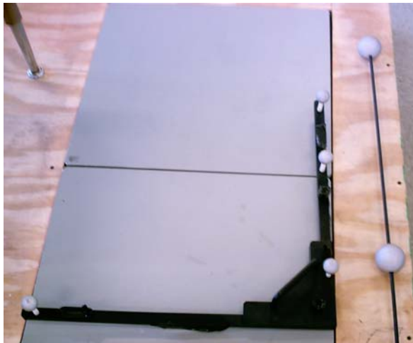
Figure 4.4. L-frame and wand used for the calibration of the Vicon™ motion analysis system.
