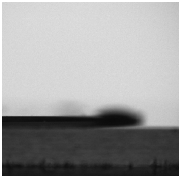
Figure 17 Image of 800 \mu L dry collagen film using the contact angle software.
