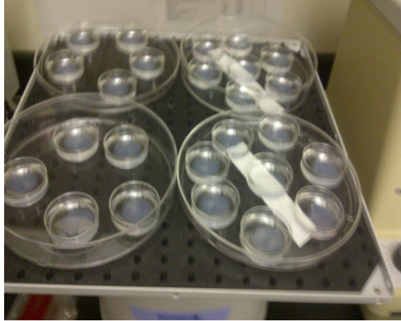
Figure 10 Rinsing of 800 \mu L collagen gels with deionized water.
