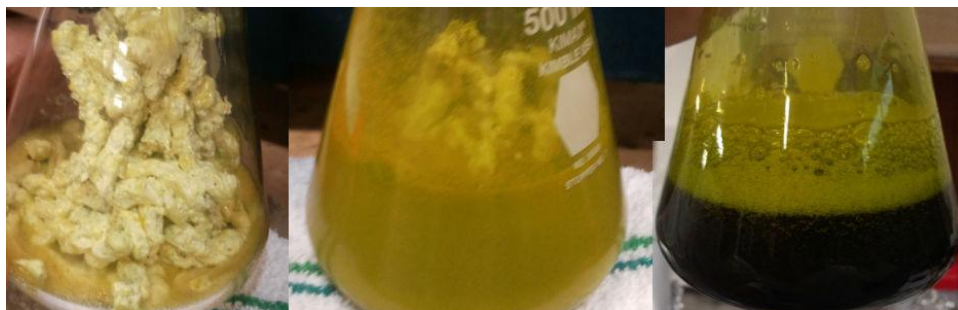
Figure 26: Supercritical Carbon Dioxide at 600 bar Açai Extract
