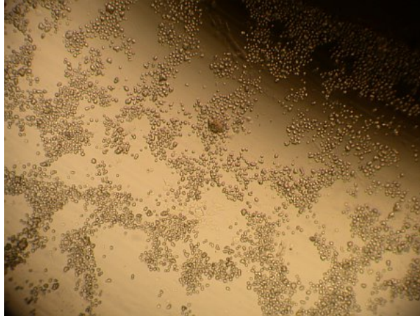
G) After 6 Cycles of 1 Minute Negative Corona Followed by 1 Minute Positive Corona
