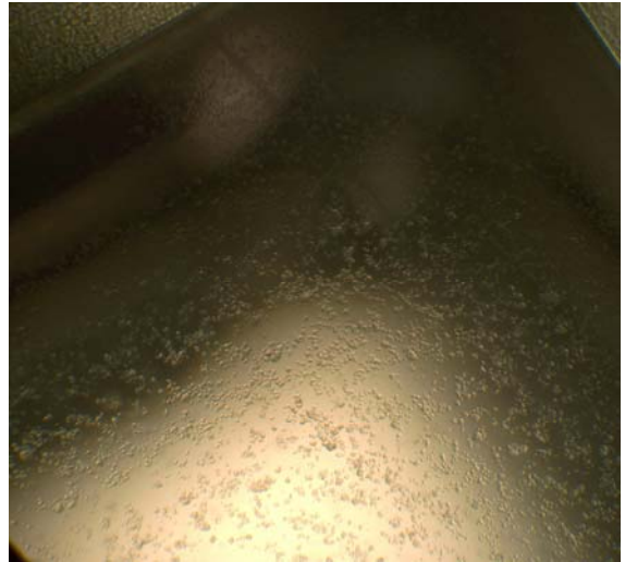
D) After 3 Cycles of 1 Minute Positive Corona Followed by 1 Minute Negative Corona
