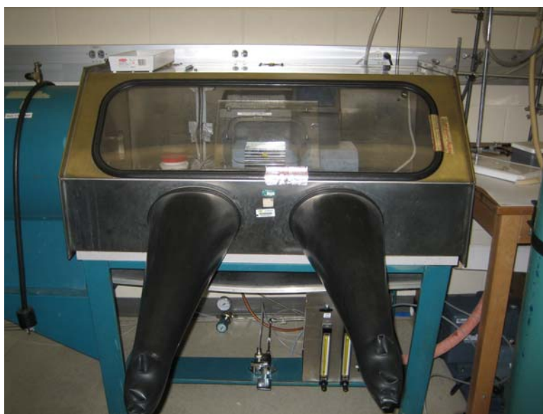
Figure 3.13: SDT-Q600 Inside an Inert Atmosphere Glove Box.
