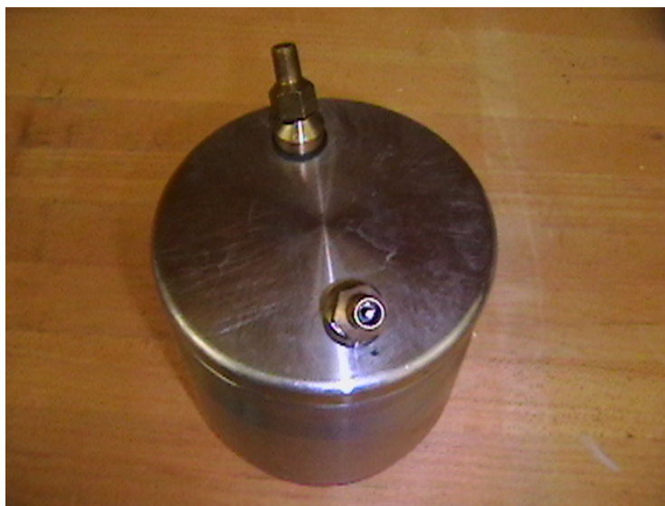
Figure 3.2: Ball Milling Bowl and the Specially Designed Lid with Schrader Valves.
