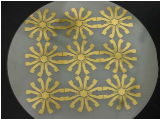
Figure 9-1. Hexagonal SAW device used for chemical and bio-sensing applications as well as materials characterization.
