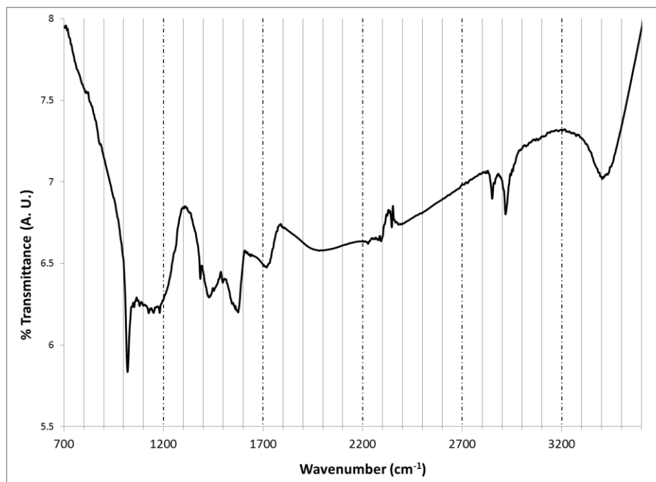
Figure 3.7 FT-IR Spectrum of rGO via L-Ascorbic Acid
