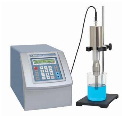
Figure 2.4 QSonica Sonicator Q500 [21]
