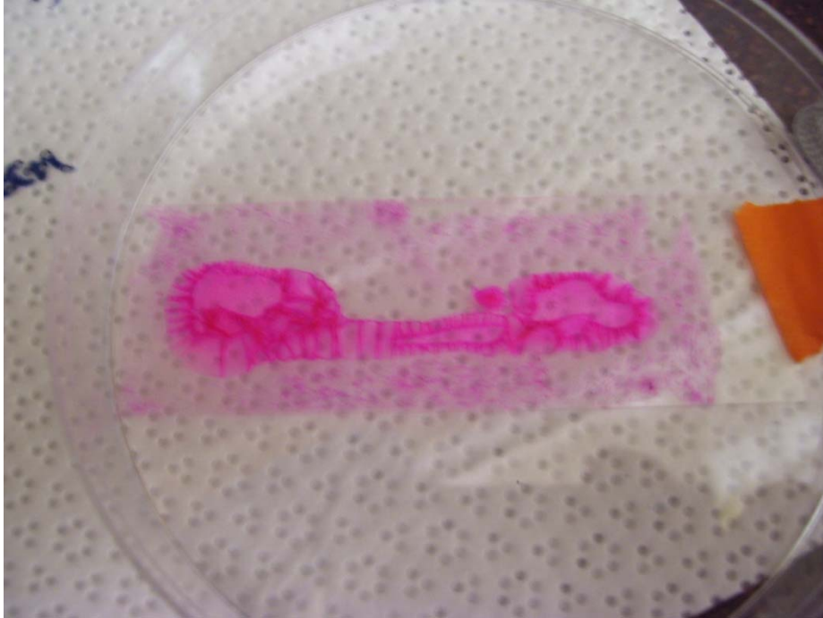
Figure 2-13: Slide with crystallized monomers (prepolymer solution) on it.
