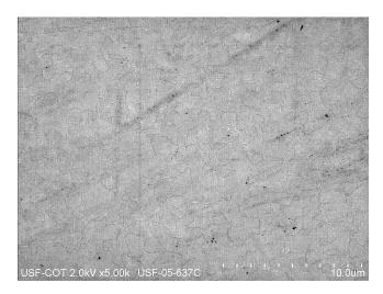
Figure 3.8 Plan-view SEM image shown at a magnification of 5.0k for a representative 3C-SiC layer grown with the no HCl process at a rate of  $\sim$ 8.6  $\mu$ m/h grown. Image courtesy of D. Edwards, USF COT.
