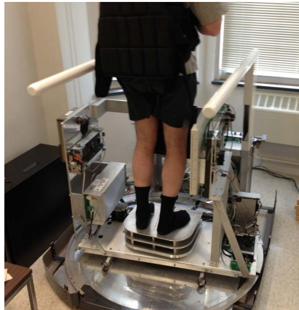
Figure 1-10 – Images of the prototype WBCT scanner with loading frame under development (top) and with subject in flexed-knee stance (bottom). The patient's knees rest against an anterior restraining plate.
