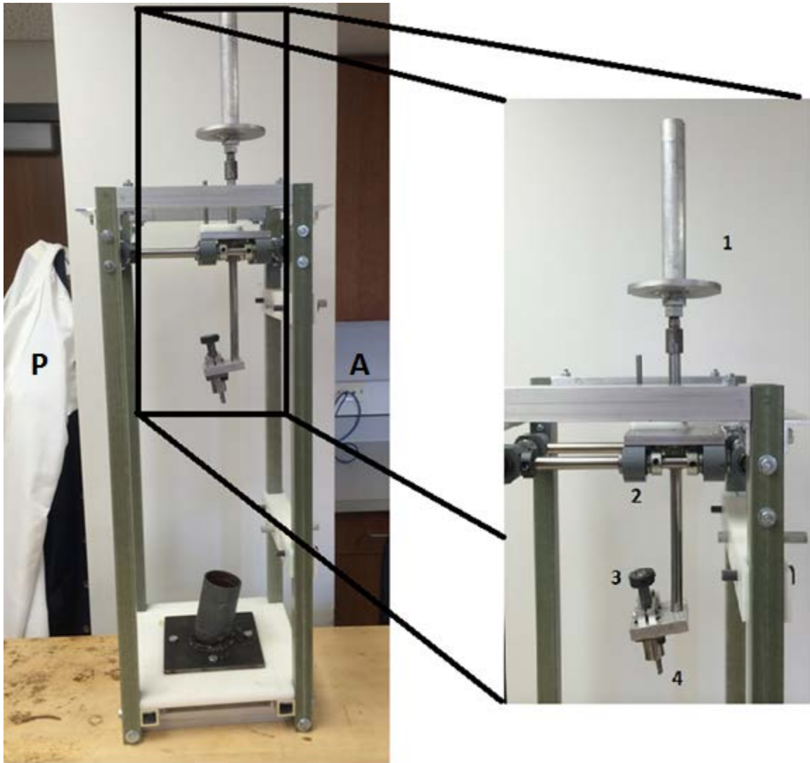
Figure 2-1 – Validation frame implementing all DoF's as designed. The position of components shown is similar to their position when attached to a knee and loaded. (left) Moveable components of the WBCT loading frame: (1) vertical load applicator, (2) transverse plane translation table, (3) axial bone rotation mechanism, (4) varus/valgus rotation mechanism. (Right) Not pictured on the right is the tibial angle fixation, which can be seen attached to the base on the left. 1
