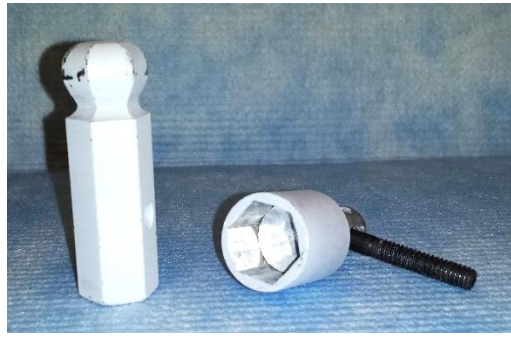
Figure 14: Hex Joint. Used to apply pure moments in axial rotation.
