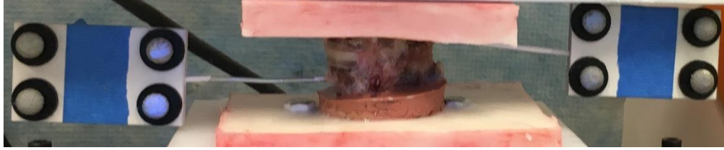
Figure 18: Reflective Marker Orientation and Attachment to Each Vertebra.
