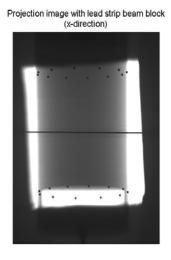
Figure 5.4: Experimental projection image using the lead strip beam block method.
