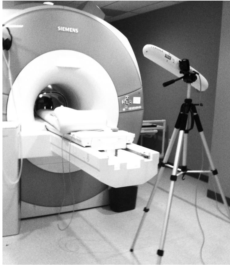
Figure 9.2. Stereoscopic camera system in position at the MR scanner.
