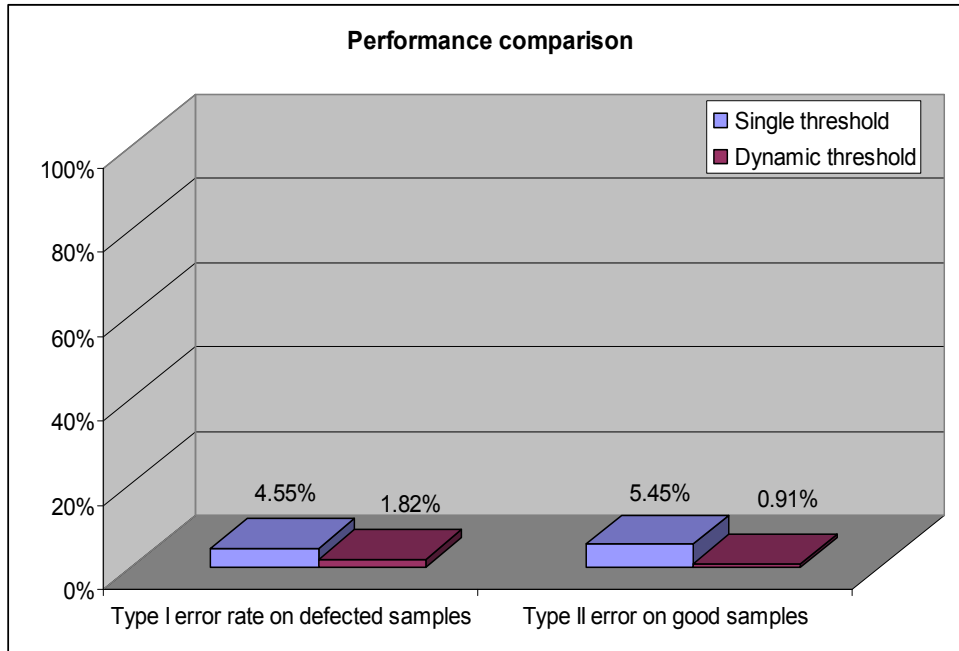
Figure 46. Performance comparison based on two test criteria between original single threshold and dynamic thresholding approaches
