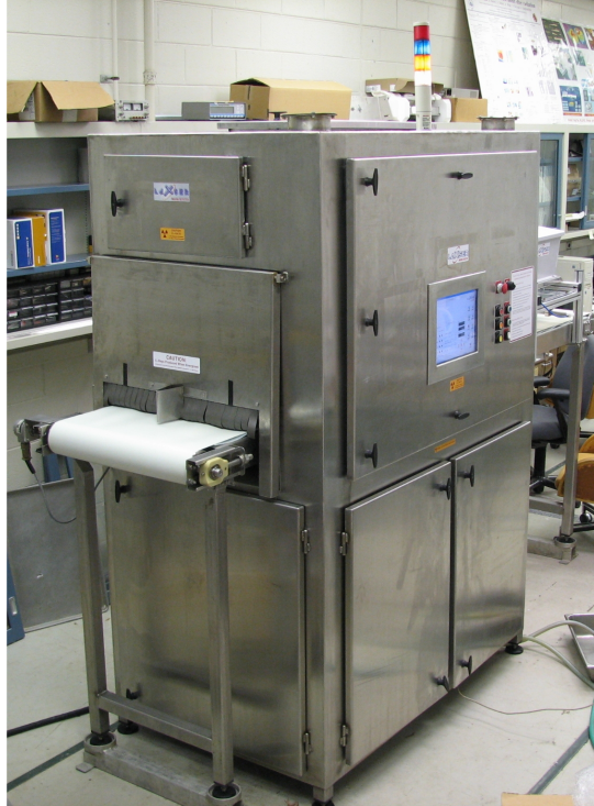
Figure 9. A snapshot of the x-ray and laser synergetic imaging detection system
