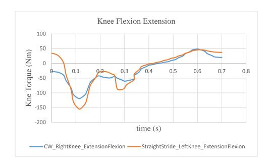
Figure 5.4: Comparison of Joint Torque Profiles for Straight Jogging Stride and Clockwise Jogging Stride Simulations
