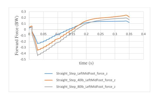
Figure 3.10: Comparison of Fore-Aft GRF for Straight Jogging Left Step Simulations with No Load, 40 lb Backpack and 80 lb Backpack
