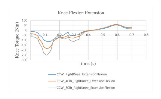
Figure 5.20: Comparison of Joint Torque Profiles for Counter Clock-wise Jogging Stride Simulations with No Load, 40 lb Backpack and 80 lb Backpack
