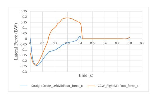
Figure 5.18: Comparison of Lateral GRF for Straight Jogging Stride and Counter Clockwise Jogging Stride Simulations
