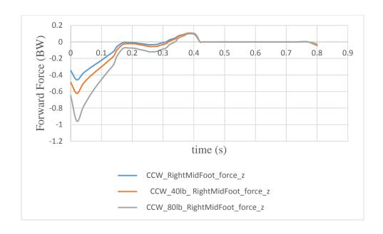
Figure 5.22: Comparison of Fore-Aft GRF for Counter Clock-wise Jogging Stride Simulations with No Load, 40 lb Backpack and 80 lb Backpack
