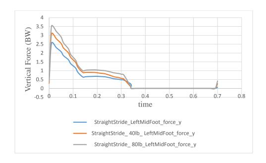
Figure 4.8 Comparison of Vertical GRF for Straight Jogging Stride Simulations with No Load, 40 lb Backpack and 80 lb Backpack
