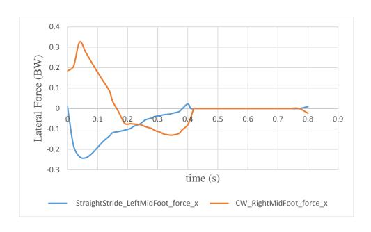
Figure 5.7: Comparison of Lateral GRF for Straight Jogging Stride and Clock-wise
