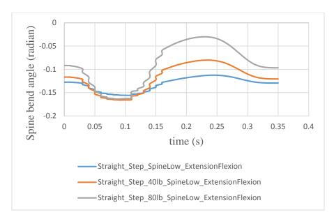
Figure 3.12: Comparison of Joint Angles for Straight Jogging Left Step Simulations with No Load, 40 lb Backpack and 80 lb Backpack
