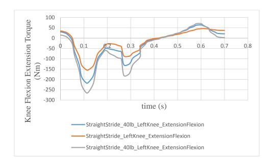
Figure 4.7 Comparison of Joint Torque Profiles for Straight Jogging Stride Simulations with No Load, 40 lb Backpack and 80 lb Backpack
