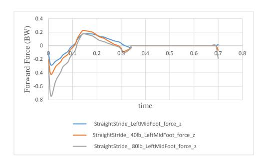
Figure 4.9 Comparison of Fore-Aft GRF for Straight Jogging Stride Simulations with No Load, 40 lb Backpack and 80 lb Backpack
