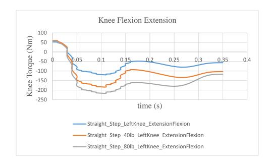
Figure 3.8: Comparison of Joint Torque Profiles for Straight Jogging Left Step Simulations with No Load, 40 lb Backpack and 80 lb Backpack
