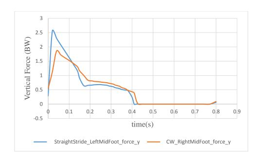
Figure 5.5: Comparison of Vertical GRF for Straight Jogging Stride and Clock-wise Jogging Stride Simulations
