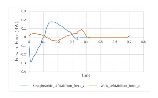
Figure 4.4: Comparison of Fore-Aft GRF for Straight Jogging Stride and Walking Stride
