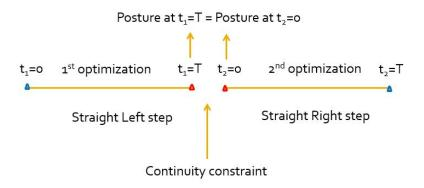
Figure 3.1 Continuity condition constraint
