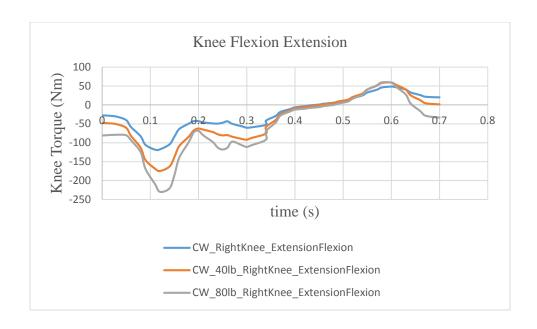
Figure 5.9: Comparison of Joint Torque Profiles for Clock-wise Jogging Stride Simulations with No Load, 40 lb Backpack and 80 lb Backpack
