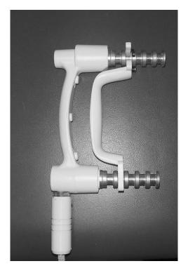
Figure 1. Modified hand grip dynamometer
