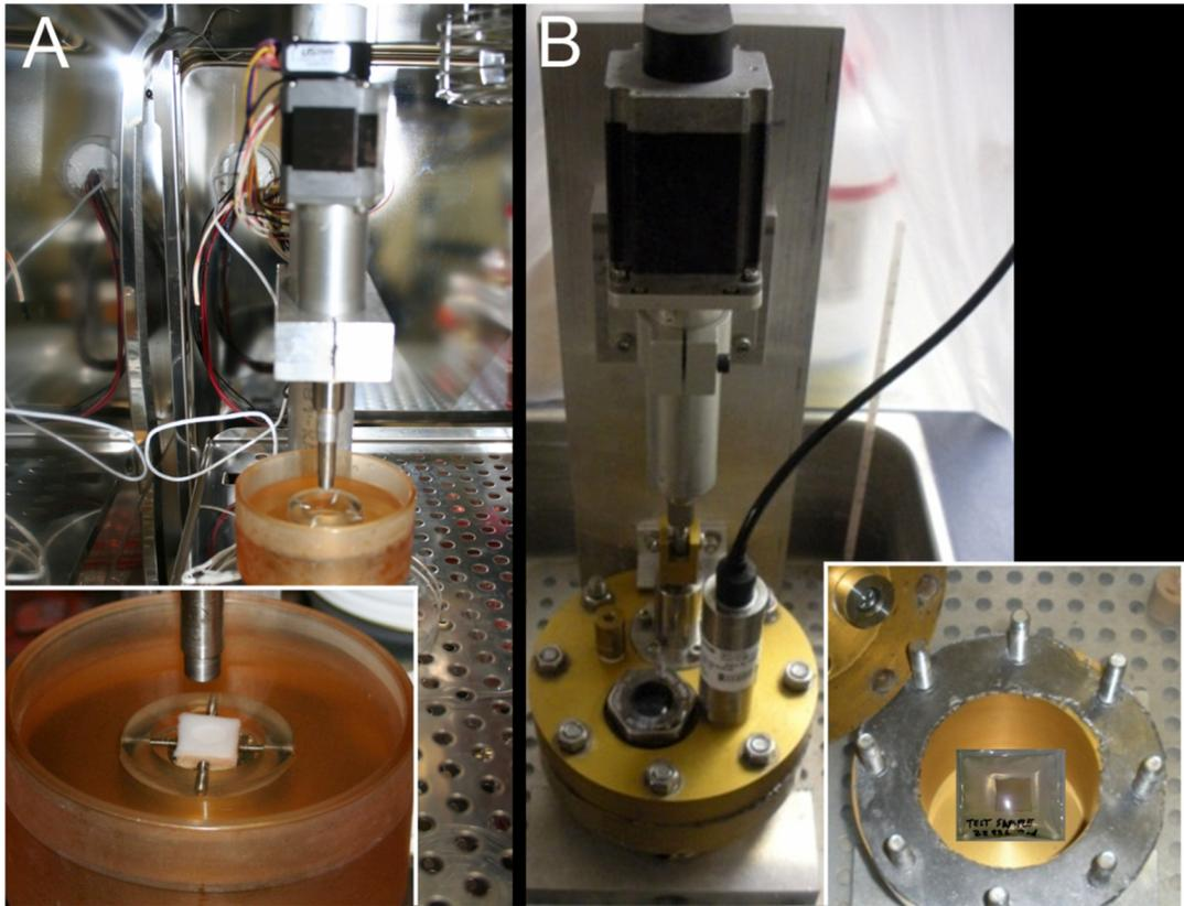
Figure 4. Mechanical loading devices. (A) Device for compressive stress shown in a low oxygen incubator. The inset shows an osteochondral explant submerged in culture medium in the housing under the compression platen. (B) Hydrostatic device shown in a water bath. The inset shows an explant sealed in a plastic bag containing culture medium. The bag is submerged under water in the unit.
