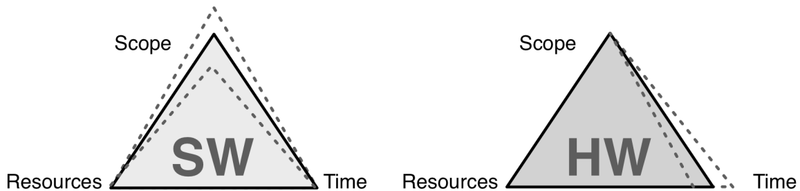
Figure 9–3: Differences in Constraint Management in Software and Hardware
