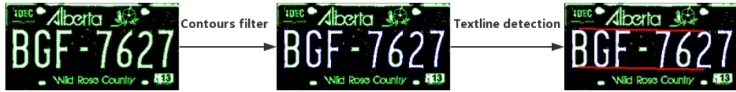
Figure 23: Procedure for contours filter and text line detection
