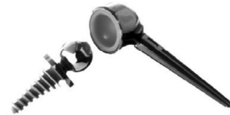
Figure 1-13 Image of Bayley-Walker RSA implant system. The several design differences from the Grammont style design are evident. The polyethylene cup is encased in metal, and the medial edge of the glenosphere does not sit flush with the glenoid bone. Taken from Ahir et al. 2004.
