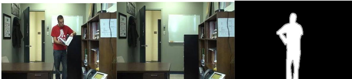
Fig 1.4: Background subtraction example for two frames of the sequence 'office' Background of the scene, and ground-truth foreground mask (source, www.changedetection.net ).
