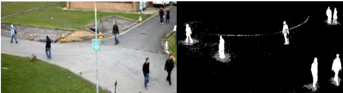
Fig 3.2 Example of Gaussian mixture Model [89]
