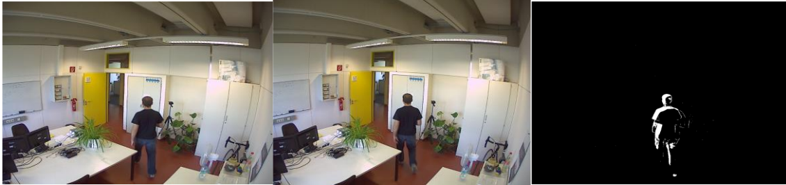
Fig 1.3: Temporal differencing. From left to right: first image of a pair containing one Moving person, second image of the same image pair, and difference mask.
