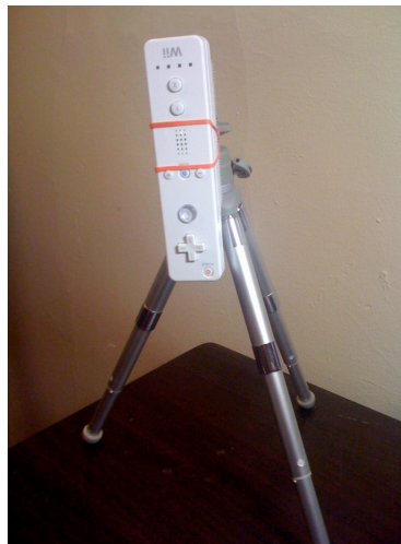
Figure 3.1 Wii Remote on tripod for IR tracking
