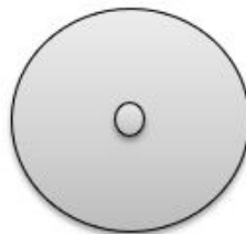
Figure 2.16: Single mode fiber
