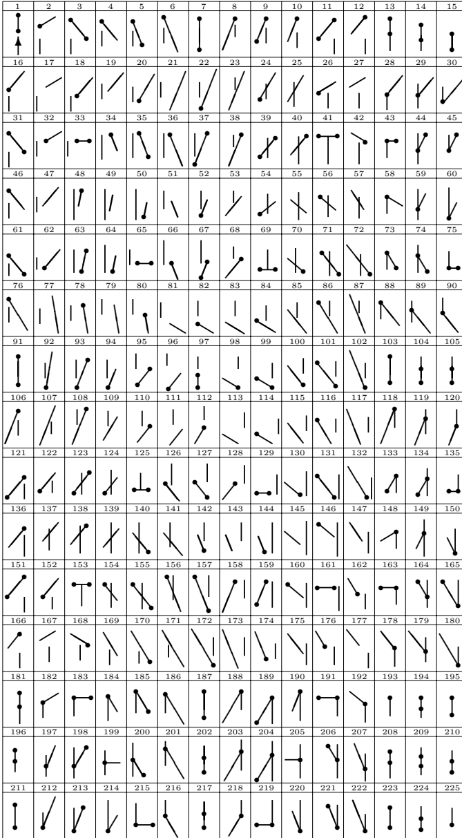
Figure 3.6: There are 225 possible two-dimensional bipartite arrangements if the two endpoints of the two intervals are distinguishable; the bulky points denote singular positions of the endpoints of the primary interval which lie on the reference system
