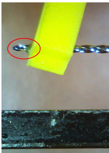
Figure 5.1 The rubber limiter is shown adjacent to the thickness reference block (1.52 mm). Accurate GT assessment was made difficult when the limiter lay at an angle to the needle. Note the liquid residue at the tip of the needle, circled in red.
