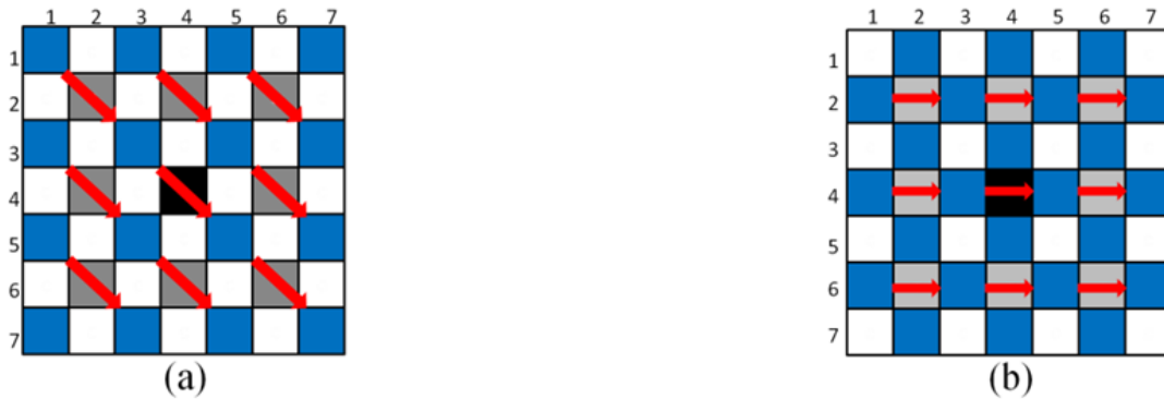
Figure 5.4. (a) 135^\circ direction gradient example. (b) 0^\circ direction gradient example. Note: the blue pixels are of known value, the black pixel is the target pixel, the gray pixels are the same type as the target pixel, and the white pixels are of unknown value.
