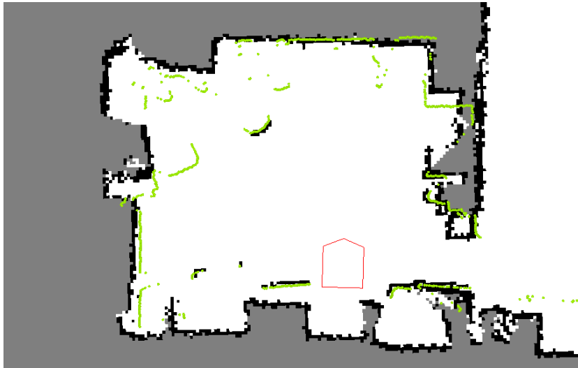
Figure 8.2: Obstacles Layer - Sensor data is shown in green
