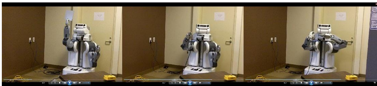
Figure 2: Robot Gesturing, (left) calibration imitation, (center) waving cord, (right) pointing at plug
