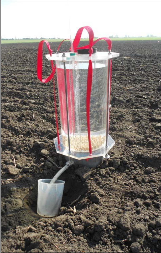
Figure 3.2. Cornell Sprinkle Infiltrometer
