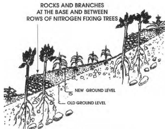
Figure 9: Buildup of terraces over time
