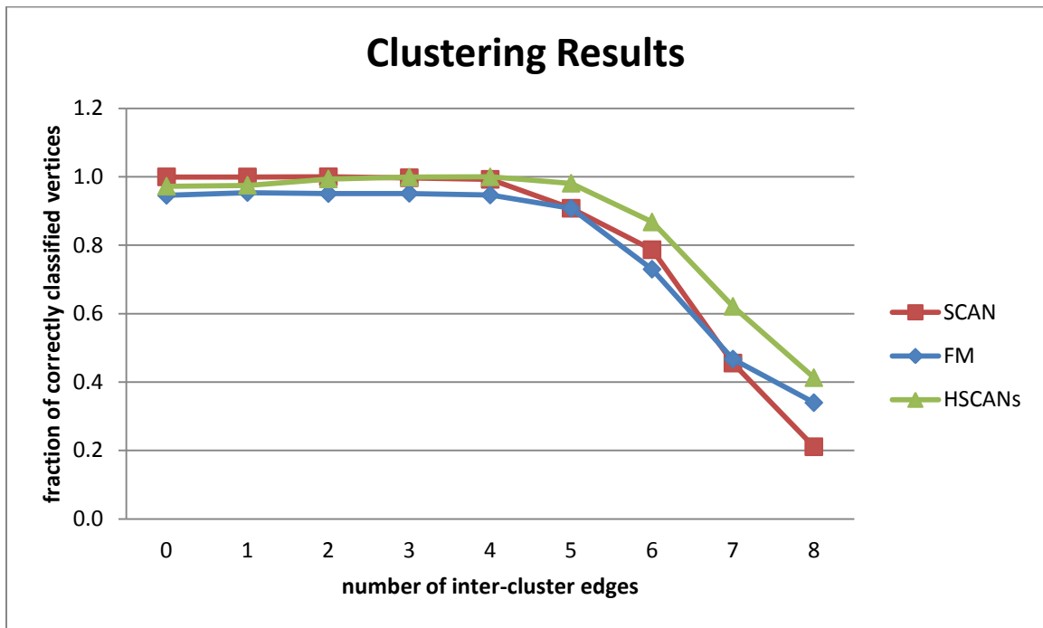
Figure 20 - Fraction of vertices classified correctly after small increase of intra-cluster weights. Every point of the chart corresponds to the average value of 100 random graphs.
