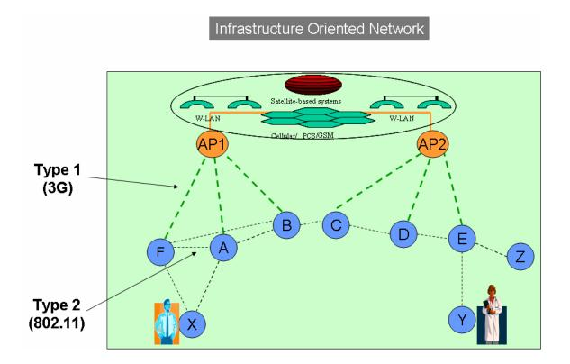
Figure 3: Use of Ad Hoc Wireless Network for Patient Monitoring
