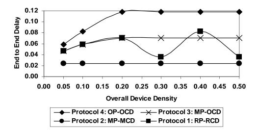
Figure 42: End-End Delays in Transmission for Uniform Device Distribution (C=0) at System Utilization = 15%
