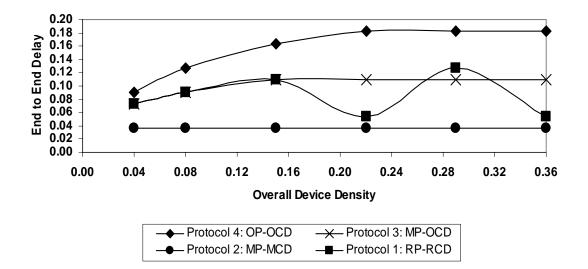
Figure 49: End-End Delays in Clustered Device Distribution (C=1, 30% of PMDs) at System Utilization = 45%
