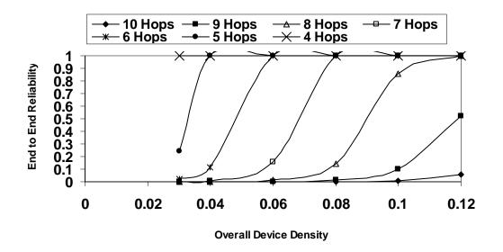
Figure 36: E-E Reliability as a Function of Variation in Device Density and E-E Hops In the Presence of Cluster = 2, Size = 40% of PMDs, Cluster Off Route of Transmission
