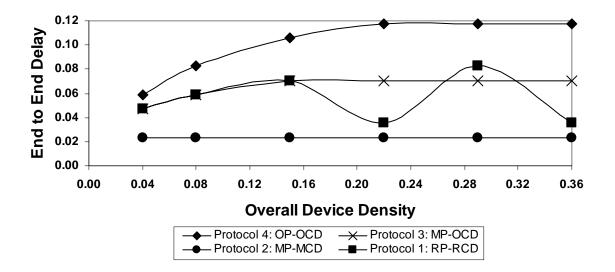
Figure 48: End-End Delays in Clustered Device Distribution (C=1, 30% of PMDs) at System Utilization = 15%
