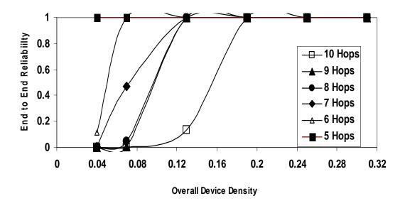
Figure 32: E-E Reliability as a Function of Variation in Device Density and E-E Hops In the Presence of Cluster = 1, Size = 40% of PMDs, Cluster Off Route of Transmission
