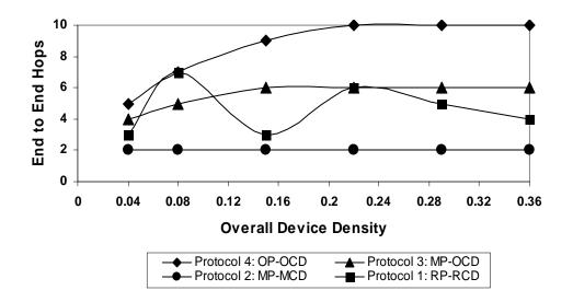
Figure 47: End to End Hops for Uniform Device Distribution, C=1, 30% of PMDs
