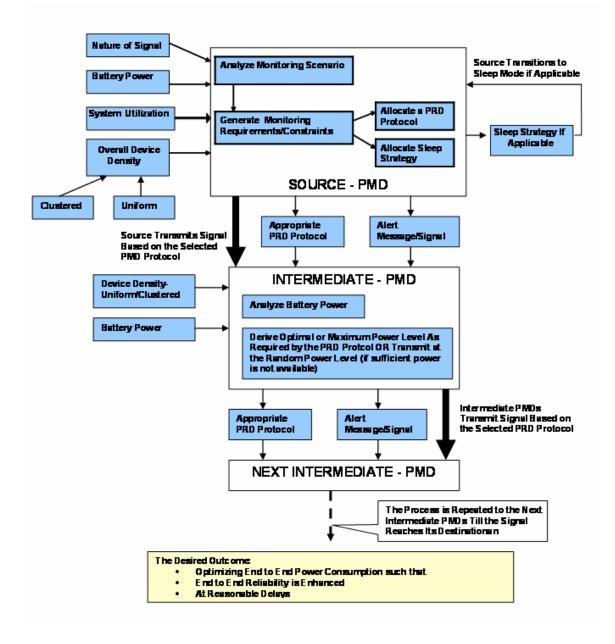
Figure 23: Process Model Underlying the PM-PRD Scheme
