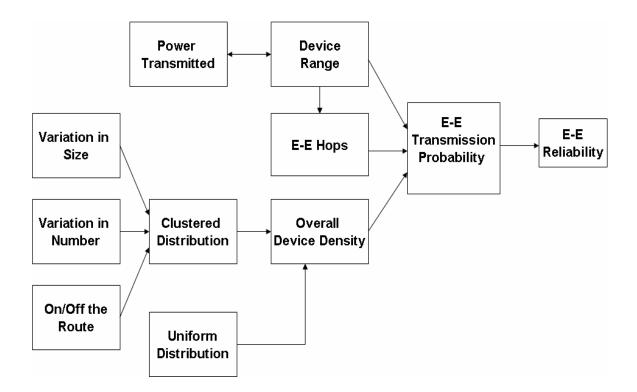
Figure 6: Parameters Impacting End to End Reliability of Transmission
