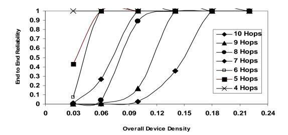
Figure 33: E-E Reliability as a Function of Variation in Device Density and E-E Hops In the Presence of Cluster = 2, Size = 30% of PMDs, Cluster On Route of Transmission
