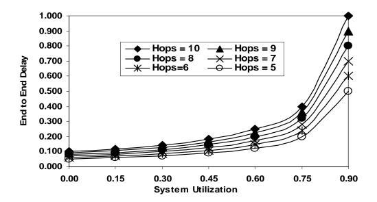
Figure 28: E-E Delays as a Function of Variation in System Utilization and E-E Hops
