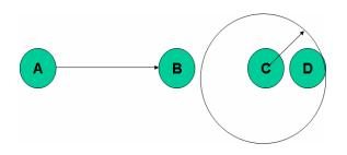
Figure 10b: Transmission from C to D at Lower Power *Reduces* Interference at B
