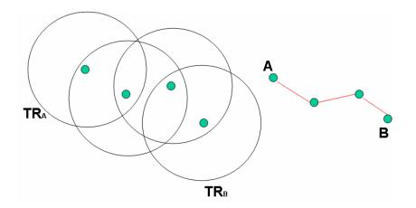
Figure 5: Multi-Hop Signal Transmission in Ad Hoc Wireless Network
