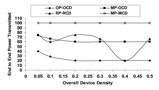
Figure 39: End-End Power Transmitted for Uniform Device Distribution, C=0
