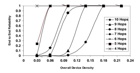
Figure 34: E-E Reliability as a Function of Variation in Device Density and E-E Hops In the Presence of Cluster = 2, Size = 30% of PMDs, Cluster Off Route of Transmission
