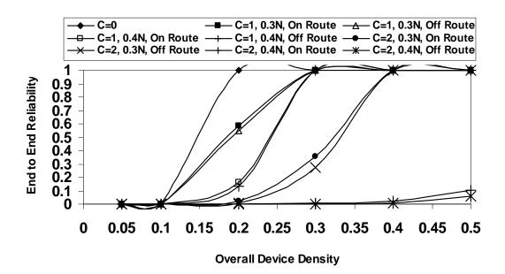
Figure 37: E-E Reliability for 10 E-E Hops and Variable Overall Device Density Due to Variations in Cluster Size, Number, and Clusters On/Off Route
