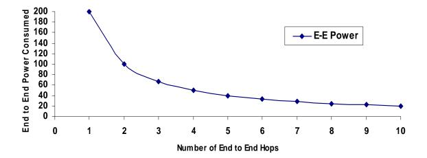
Figure 26: E-E Power Usage as a Function of Variation in E-E Hops
