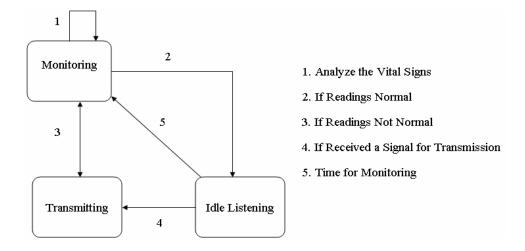
Figure 11: Monitoring Device's State Model
