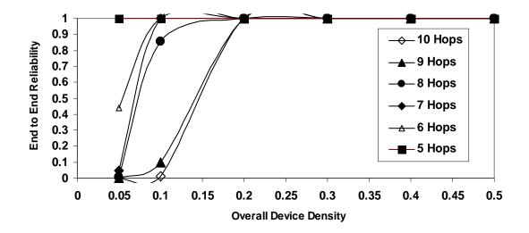
Figure 27: E-E Reliability as a Function of Variation in Device Density and E-E Hops
