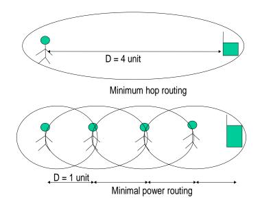
Figure 8: Minimal Delay Transmissions vs. Minimal Power Transmissions
