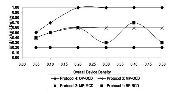
Figure 44: End-End Delays in Transmission for Uniform Device Distribution (C=0) at System Utilization = 90%
