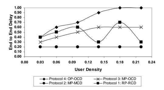
Figure 56: End-End Delays in Clustered Device Distribution (C=2, 30% of PMDs) at System Utilization = 90%
