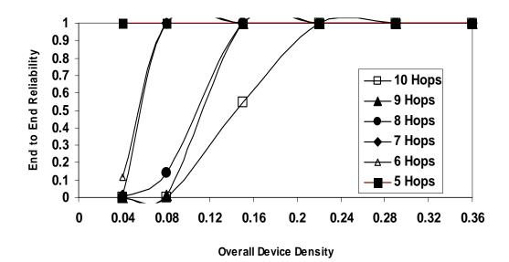
Figure 30: E-E Reliability as a Function of Variation in Device Density and E-E Hops In the Presence of Cluster = 1, Size = 30% of PMDs, Cluster Off Route of Transmission
