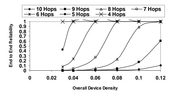
Figure 35: E-E Reliability as a Function of Variation in Device Density and E-E Hops In the Presence of Cluster = 2, Size = 40% of PMDs, Cluster On Route of Transmission
