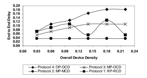
Figure 55: End-End Delays in Clustered Device Distribution (C=2, 30% of PMDs) at System Utilization = 45%
