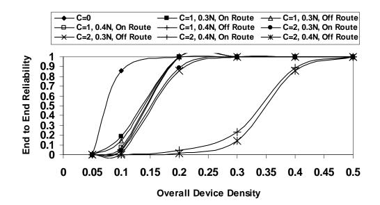
Figure 38: E-E Reliability for 8 E-E Hops and Variable Overall Device Density Due to Variations in Cluster Size, Number, and Clusters On/Off Route
