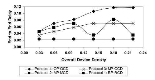
Figure 54: End-End Delays in Clustered Device Distribution (C=2, 30% of PMDs) at System Utilization = 15%
