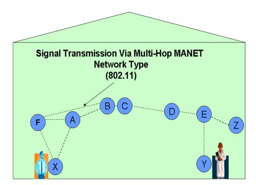
Figure 24: The Network Model - Transmission from X to Y via A-B-C-D-E
