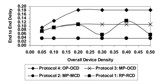
Figure 43: End-End Delays in Transmission for Uniform Device Distribution (C=0) at System Utilization = 45%
