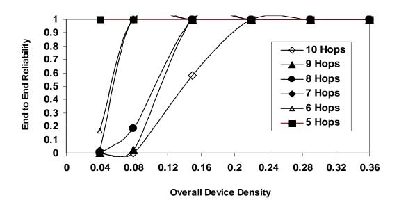
Figure 29: E-E Reliability as a Function of Variation in Device Density and E-E Hops In the Presence of C=1, 30% of PMDs, Cluster on Route of Transmission
