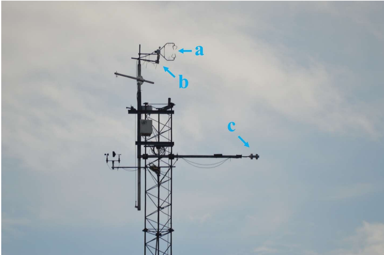
Figure 2.2: View of the instrumentation mounted at the top of Sunset Tower as seen from the West. The (a) 3D sonic anemometer, the (b) infrared gas analyzer, and the (c) net radiometer are pictured here.
