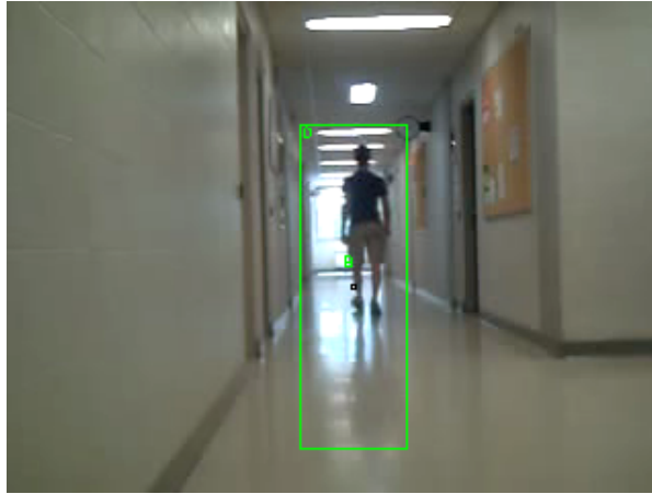
Figure 2.3: Poor image quality. Notice the low-resolution and blurred appearance of the walking man.
