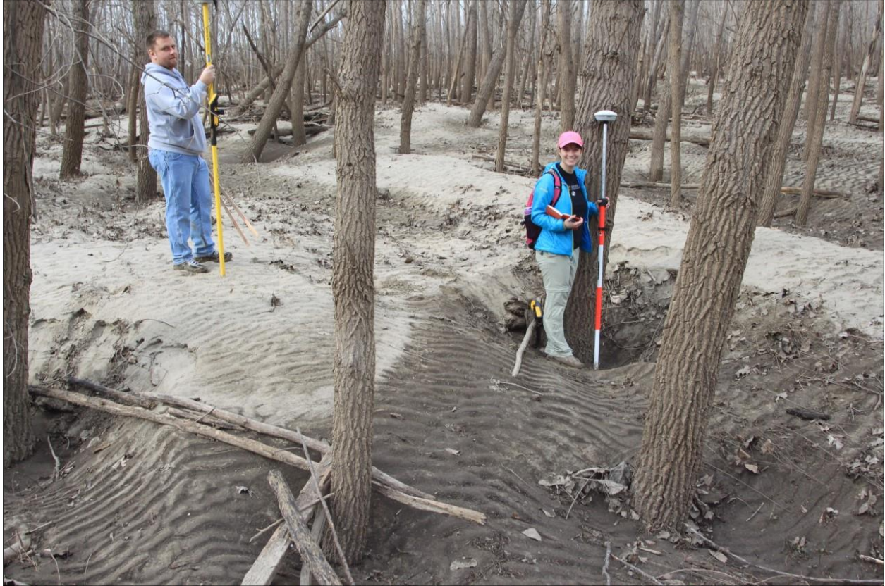
Figure 13: Scour and aggradation within meters of each other due to microtopography on North Wilkinson Island.
