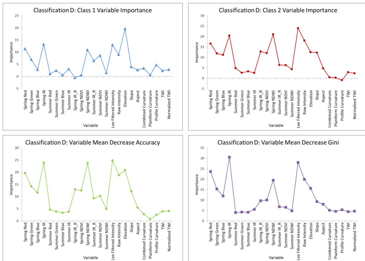
Figure 5.6 Four measures of variable importance for Classification D: 1) Class 1 (Forested Wetland) Marginal Importance; 2) Class 2 (Forested Upland) Marginal Importance; 3) Mean Decrease in Accuracy; and 4) Mean Decrease Gini Coefficient
